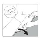
Place the first plank of the new row with the tongue side at an angle against the groove side of the plank in the
